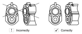
Make certain that the bushing (64) is timed correctly. Screw the bushing all the way in and then back it off to the first notch in the bushing. Recoil spring housing (63) must be engaged into the notch in the bushing.
